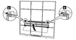
Reinstall the air filter. (Refer to step 6 in "Cleaning the air filter".)
