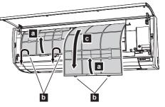
Filter holder and air cleaning filter are attached on the rear side of the air filter. Remove them from the air filter by unlatching each corner of the filter holder a.
